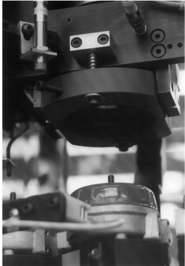
Figure 4: Coupling to motor from above using a collet.
